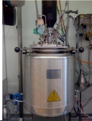
20-L autoclave vessel 150-250°C
